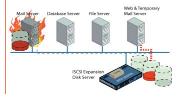
Although RAID-1 can be used across two drives inside an application server, it does little good if the server catches fires, gets wet or simply malfunctions. Having a mirrored copy on a separate disk server, ideally in a different room, increases protection levels and enables you to recover the data by simply connecting a replacement machine to the disk server and reassigning the critical volumes. It's just like rebooting the original application server after an unexpected outage.
