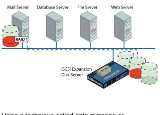
Using a technique called data mirroring or RAID-1, each time an application saves data to disk, the host operating system transparently stores the data on a local disk volume as well as
